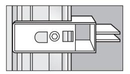
Do not remove the installation supports from the appliance doors. They will be used later in the installation niche.
